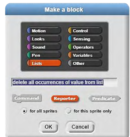
Here we define the name of the new block, its category, and whether it's a command, function, or predicate.
