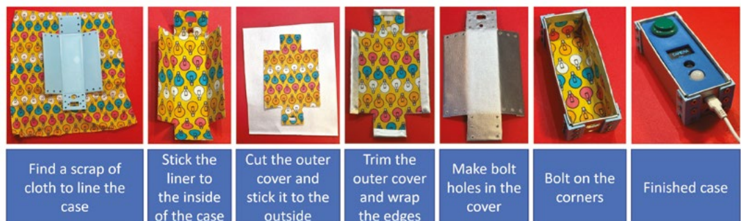
Figure 4 ♦ This version of the case design has bolt supports for covers on the end panel for the USB and tripod holes. The cover wasn't added to the finished case because it didn't seem to need them
