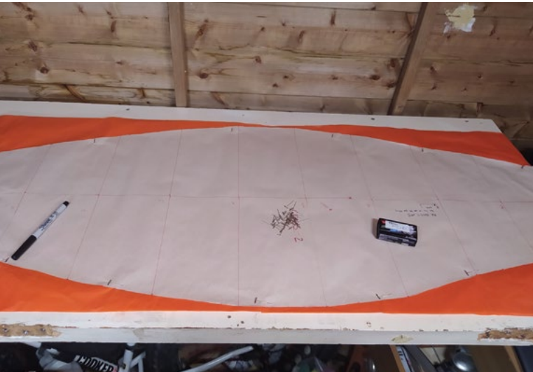
Figure 3 ⬆ For all the balloon designs, we cut the gore panels by pinning the pattern to a stack of six sheets of tissue paper
