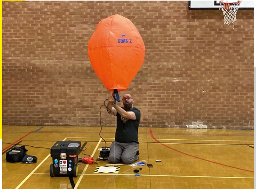
Figure 1 ⬆ The CDAS-2 balloon filled with hot air using an electric heat gun, ready to take flight
