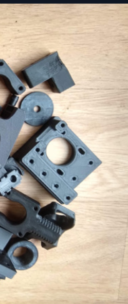
Left ← This is most of the printed parts for a Voron 0.1 – yes, they take a long time to print
