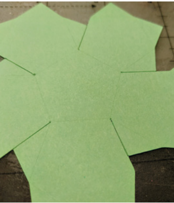
Figure 11 ♦ Cutting and scoring card using different settings for different paths in the design
