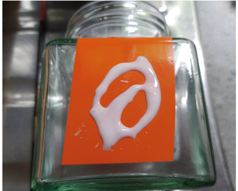
Figure 3 ♦ A glass jar is masked with a vinyl cut and the Armour Etch is applied in an even coat
