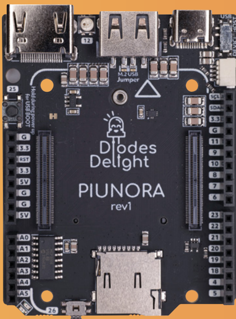
Below The final production version of the Piunora dev board, ready for a Compute Module 4 to be mounted on top
