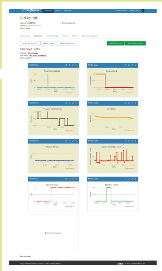
Left Your IoT network gathers data including temperature, humidity and barometric pressure
