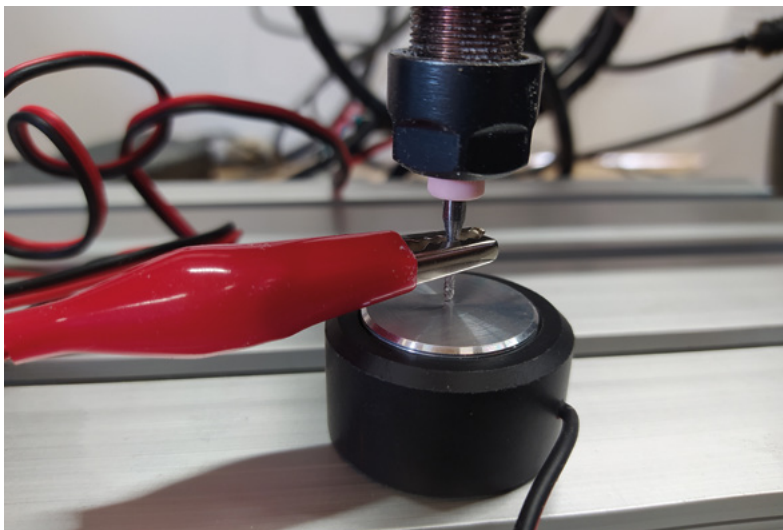
Figure 4 ◆ If you are using a conductive material, you can place your Z axis probe upside down and probe directly onto the material
