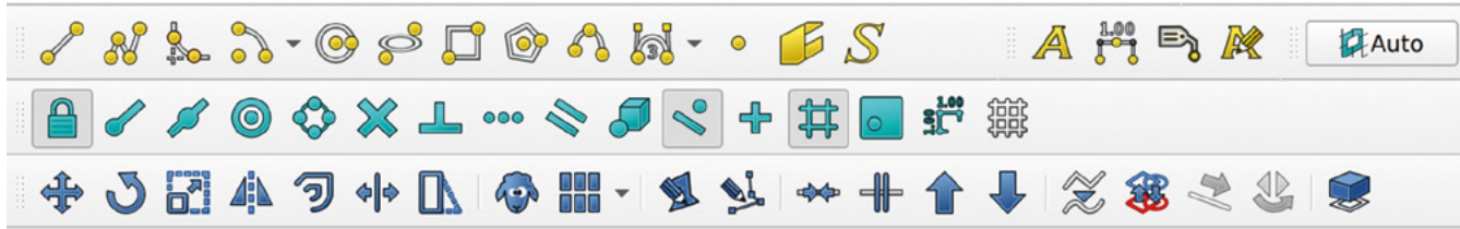
Figure 8 ■ Some of the tool icons on the Draft Workbench: top row drawing tools, middle row snap options, and lower row includes array tools
