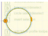
Figure 5 ♦ Adding tabs to profile toolpaths means that the work won't become loose, and is held securely throughout the machining operation
