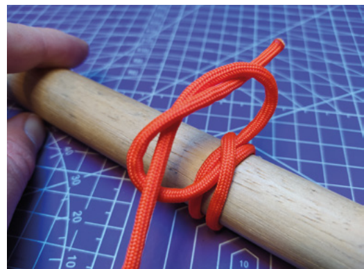
Figure 7 ♦ Forming the first half of the square knot
