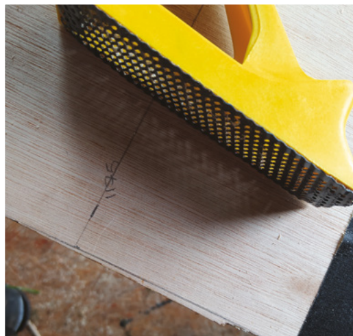
Above ♦ This little Surform tool was really handy in finishing curves and bringing internal components for the boat to fit
