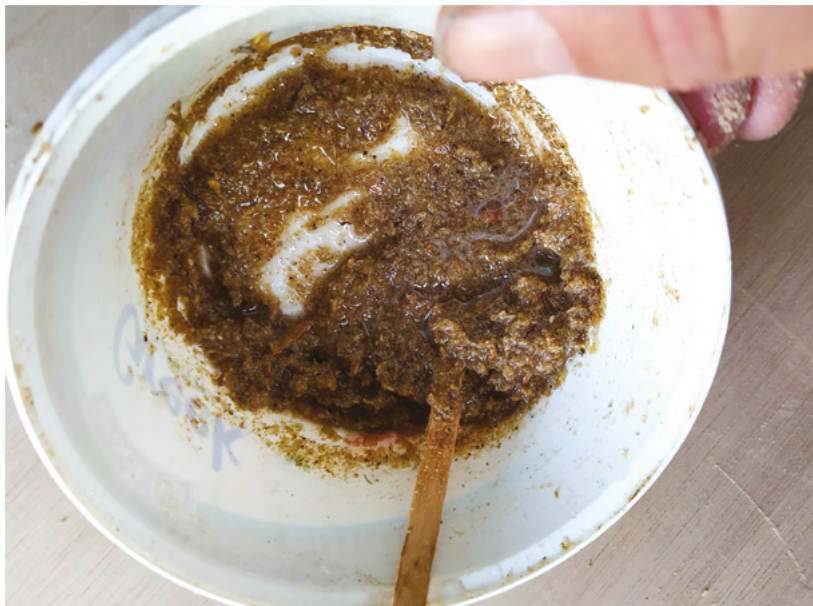
Above ♦ Using sawdust to thicken the epoxy worked, and it was free. However, it's hard to get a perfect fillet finish, so I would explore different fillers next time
