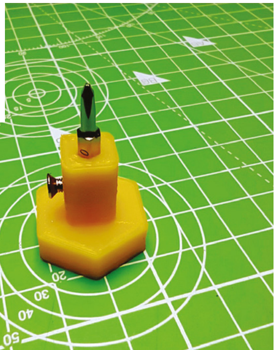
Figure 9 ♦ A simple stubby tool to hold common 4mm screwdriver bits
