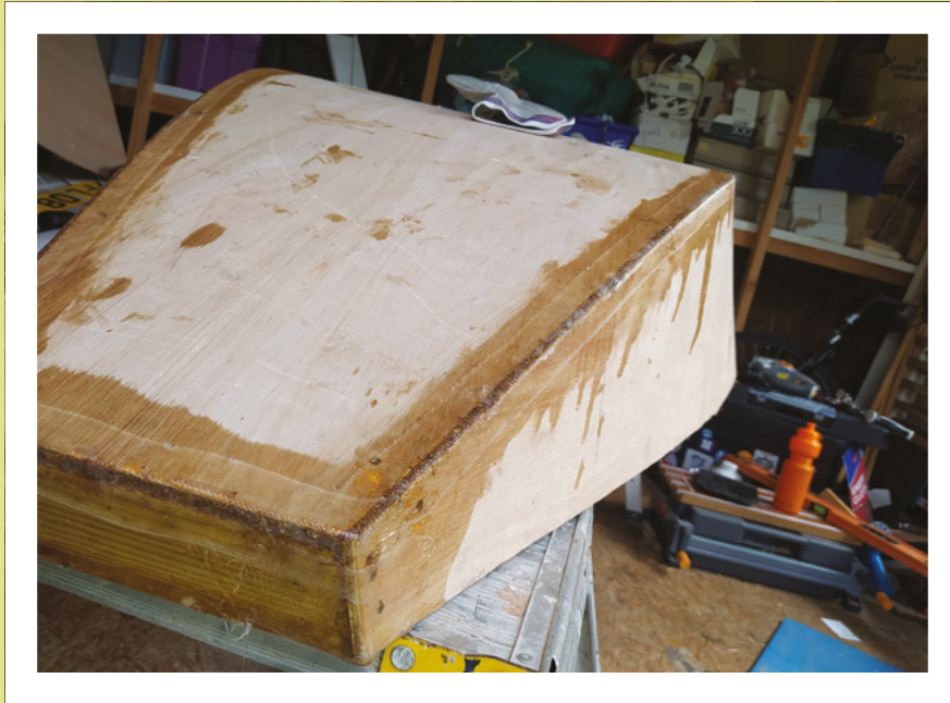
Above ♦ Applying the fibreglass tape over the filleted seams, and applying unthickened epoxy to 'wet out' the cloth
