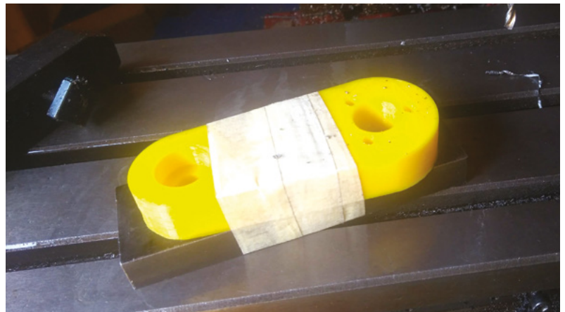
Figure 7 ♦ Vee blocks and clamps are very useful engineering items, and 3D-printed plastic ones are useful in some circumstances. The ability to make matching multiples affordably is a bonus
