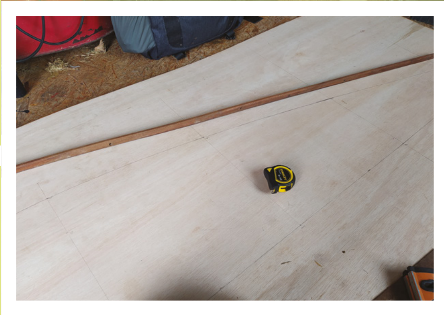
Left ♦ You may have to think creatively to work out ways to draw or 'loft' all the curves of the design
