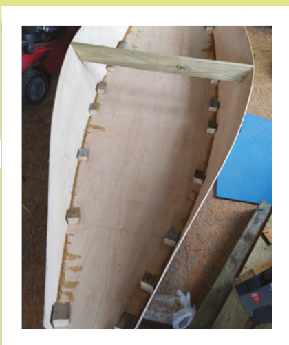
Below ♦ Once the sides, base, and stern transom are tacked together with blocks, you get your first sense of the size and shape of the boat
