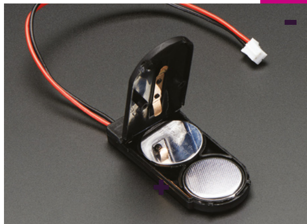
Left ◊ Coin cell battery packs – such as this one from Adafruit – are small and great for projects that don't demand lots of current
