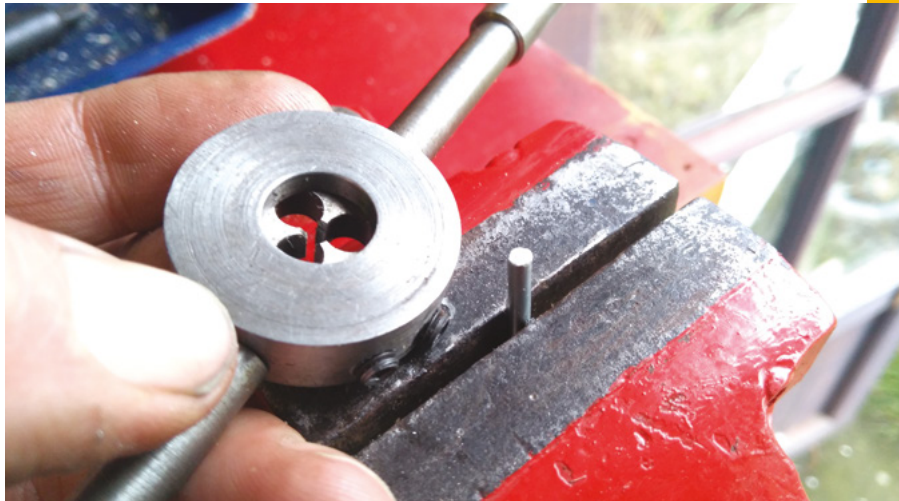
Figure 3 Using an M3 die in die holders to cut a thread into a short stud; similar to tapping an internal thread, the die must be kept horizontal in relation to the workpiece
