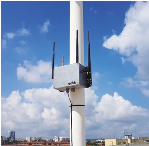
Above ◆ Mounting your gateway outside can increase the range by miles. This example from Sixfab ( hsmag.cc/3orDvd ) is powered by Raspberry Pi
