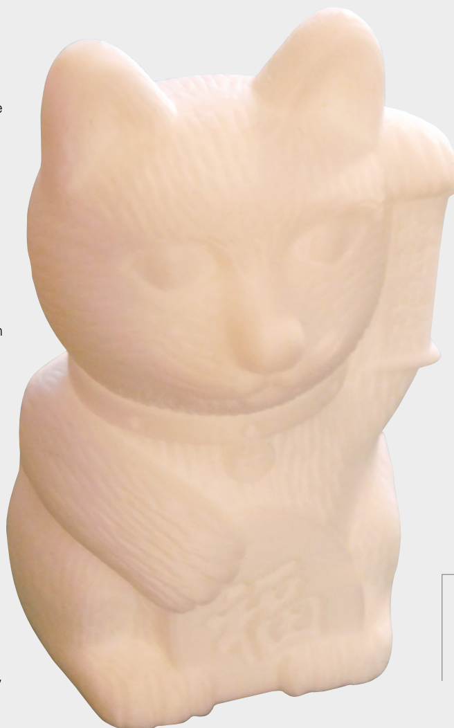
Left ♦ The first print from this printer came out well, with the only defect being a tiny amount of stringing between the ears
