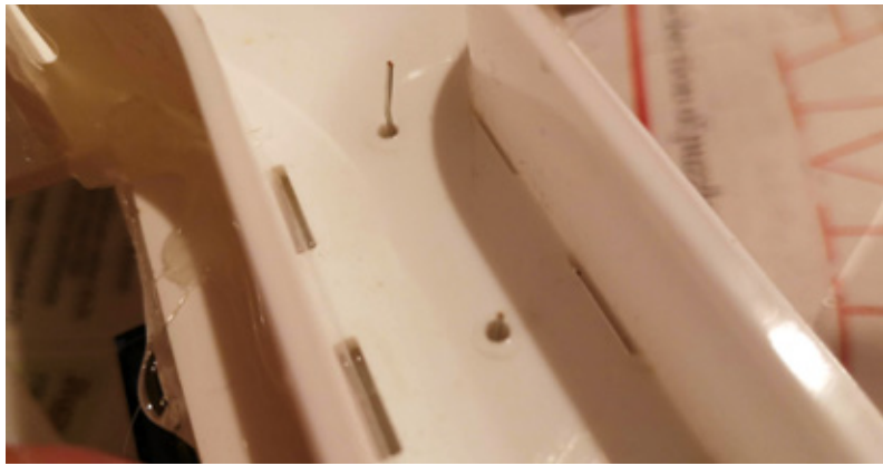
Below ♦ The pin mechanism for releasing one brick at a time
