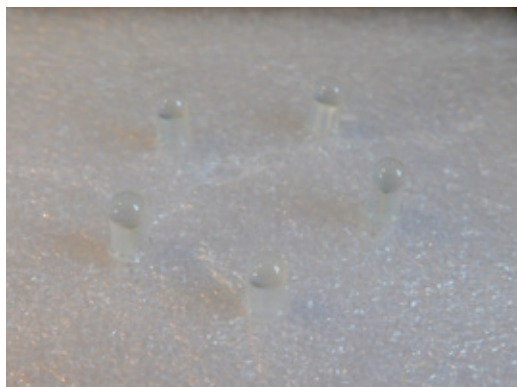
Above ♦ The LEDs held in place on foam, before committing them to the casting
