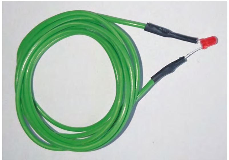
Figure 1 This is the simplest of NFC examples – just wire and an LED
