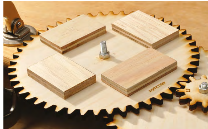
Above Boost turntable height and keep it flat and level with four plywood spacers
