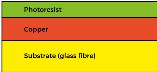
Figure 6 ♦ Layers of pre-sensitised PCB
