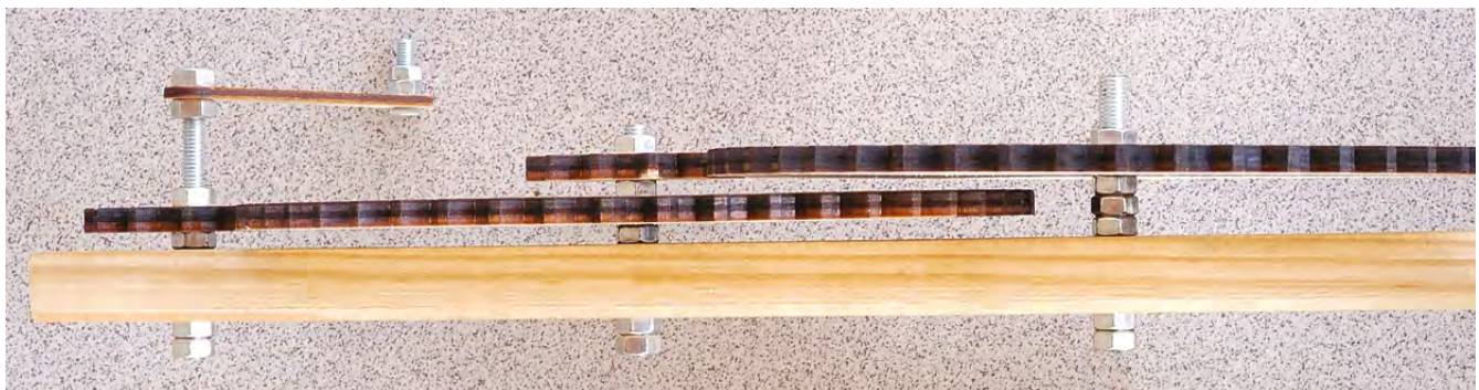
Below Side view showing vertical orientation of the gears. The large gear on axle 3 rests on three M6 nuts
