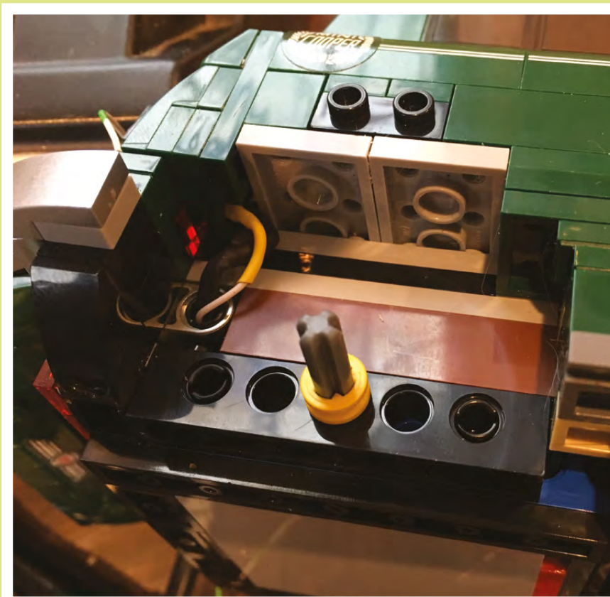
Left ♦ Wiring to the rear wheels comes via the spare wheel compartment
