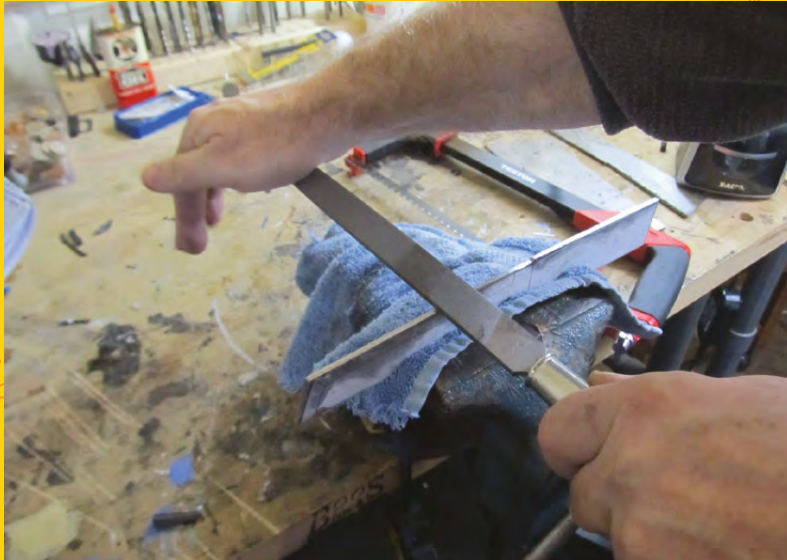
Above ♦ Finish shaping the knife with a mill file
