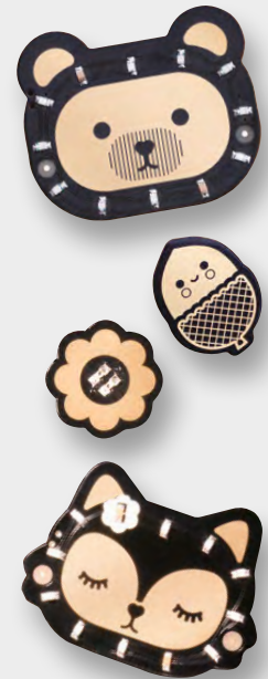
Above ♦ Each badge features twelve LEDs of various single colours that can be lit in twelve preset patterns or your own custom creations
