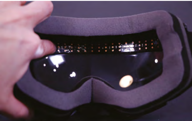
Above ♦ The NeoPixels should leave enough space to see properly
