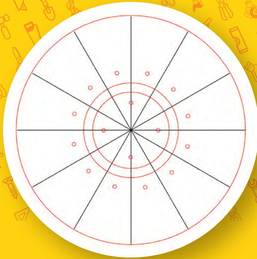
Above To keep things symmetrical, we decided to use more screws than needed, with one between every hour on the outside ring and just four on the inside circle
