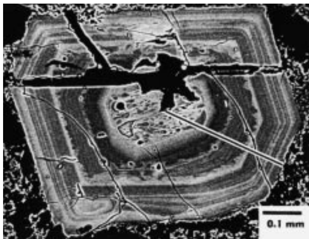
FIGURE 8. BSE photograph of plagioclase crystal SH80-D. The line shows the location of the PIXE measurement.
