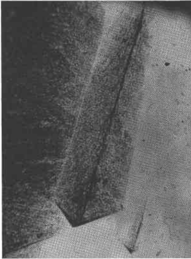
FIG. 5. Coating formation in the form of "fish bones." Original magnification on photograph reduced \frac{1}{2} on reproduction.
