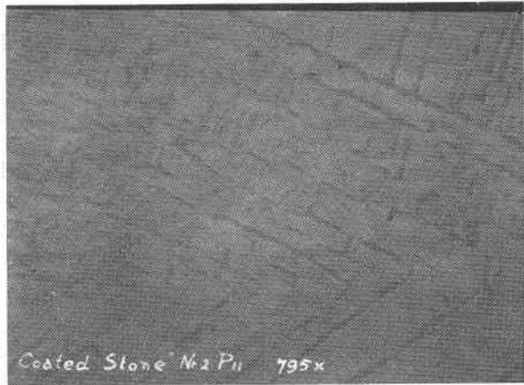
FIG. 6. Example of a regular string formation. The strings mostly include an angle of 60^\circ . This picture shows, however, also strings which include an angle of about 80^\circ . Original magnification on photograph reduced \frac{1}{2} on reproduction.
