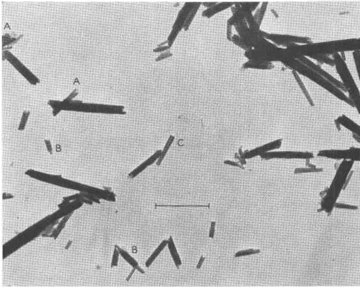
FIG. 3. Halloysite (metahalloysite) from Real County, Texas. (A) Oblique view of end section; (B) double tubes (tube in tube); (C) split and partially unrolled tube.
