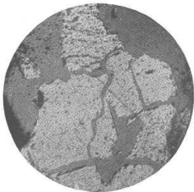
Figure 11. Angular fragments of arsenopyrite in quartz with but slight corrosion. Stannite-wolframite ore, East Pool mine, Cornwall, England. Mag. 36X.
