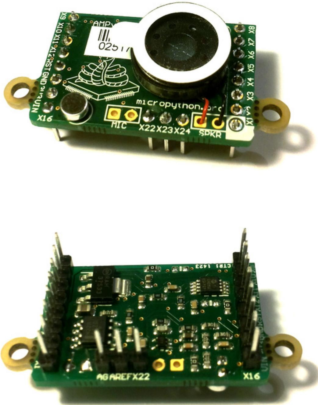
The following video shows how to solder the headers, microphone and speaker onto the AMP skin. For circuit schematics and datasheets for the components on the skin see *The pyboard hardware*.
