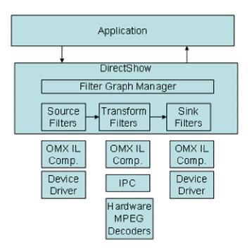
As the diagram above depicts, a multimedia application is abstracted from the underlying hardware via the DirectShow Filter Graph which is constructed by the Filter Graph Manager. Filters in this system abstract I/O device drivers and transforms(such as codecs). These Filters are connected using Pins. It is the underlying Filter interface that this paper will map to OpenMAX IL component interface so the capture devices, decoders, and rendering interfaces are abstracted in an OS independent way.
