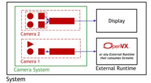
Figure 2. An example Camera System with Devices, Streams and Cameras
