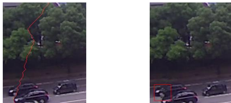
(a) Seam passes through the moving object (b) Deformation of the moving object
