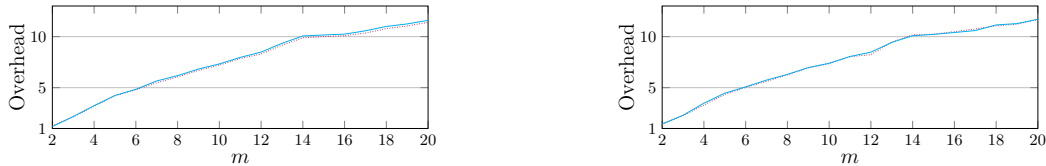
Fig. 4: The left diagram shows the bandwidth overhead of the polytuple plugin offline phase compared to classical SPDZ-like protocols for the computation of x_0 \cdots x_{m-1} . The right diagram shows the corresponding runtime overhead. For the blue line we used the LowGear offline protocol [KPR18], for the red dotted line the MASCO protocol [KOS16].
