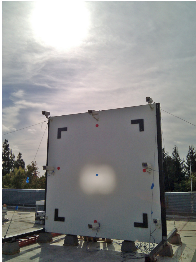
The test target with mounted cameras. Although this target has 8 cameras, only 4 were used at a time.
