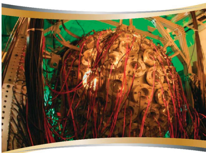
Detector for Advanced Neutron Capture Experiments at Los Alamos Neutron Science Center. (Photo provided by NNSA)
