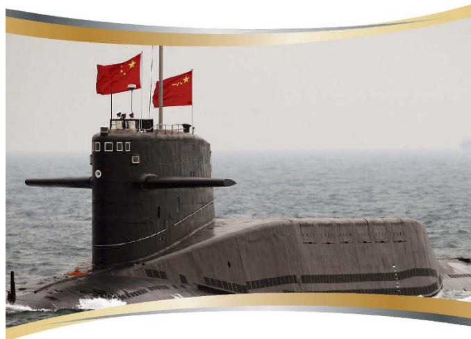
A JIN-class Type 094 ballistic missile submarine. (Photo by the People’s Liberation Army-Navy)
