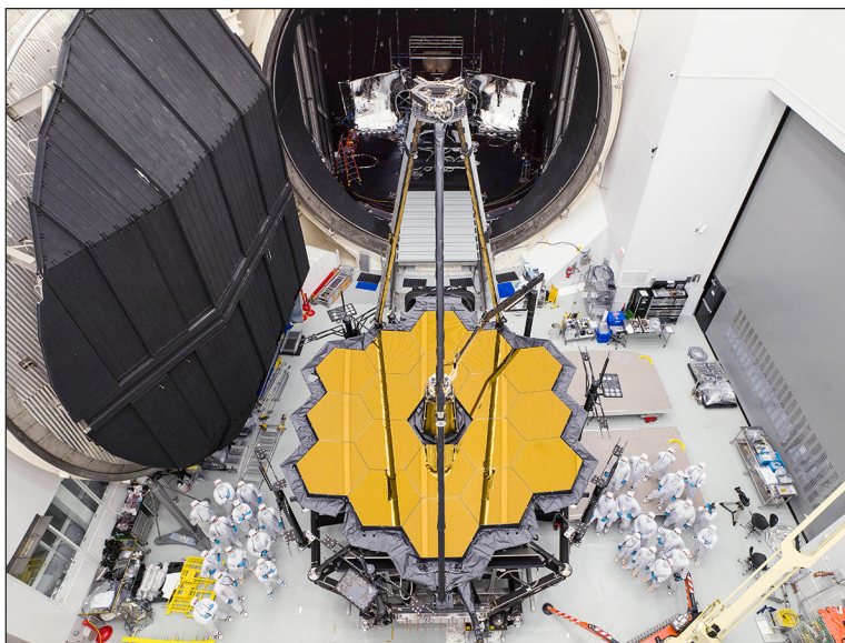
Figure 3: Optical Telescope Element and Integrated Science Instrument Module (OTIS) Emerging from Thermal Vacuum Testing Chamber
