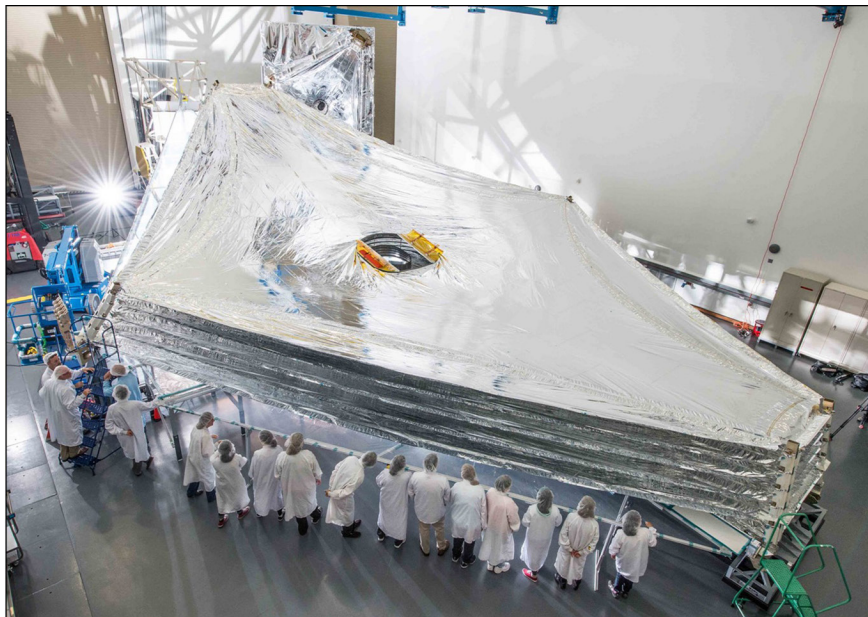
Figure 6: James Webb Space Telescope's Sunshield Template Layers
