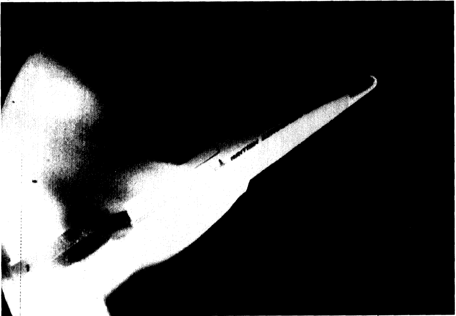
Figure 8.2: Reentry Test on a Model of HOTOL in The Australian National University T-3 Shock Tunnel
