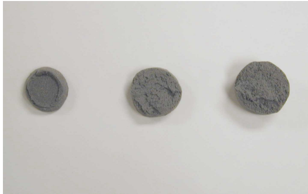
Figure 2.9. Interior of HTPB0 propellant specimens immersed for 1 year in deionized water. Specimens were sliced to reveal interior. Left to right: Immersed at 5°C, Immersed at 20°C, Immersed at 29°C. The 5°C specimen is sponge-like on the edges and remained hard inside. The hard area is 11.9 mm diameter (the original specimen diameter was 14 mm). The 20°C and 29°C specimens are sponge-like throughout.
