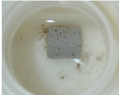
Figure 2.10. An immersed HTPB0 specimen after 1 year. Dark areas are material that appeared in the container, presumed to be evidence of biological activity. Some specimens showed no visible material. The two white areas are reflections. This study did not attempt to measure or control biological conditions
