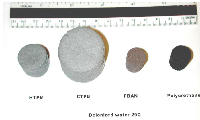
Figure 2.7. Wet solid propellant specimens after 3-month immersion at 29°C in deionized water. Left to right: HTPB, CTPB, PBAN, PU.
