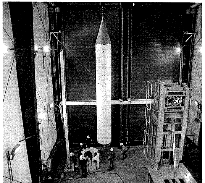
Simulated Strategic Target System missile placed on launch stool during missile checkout procedures
