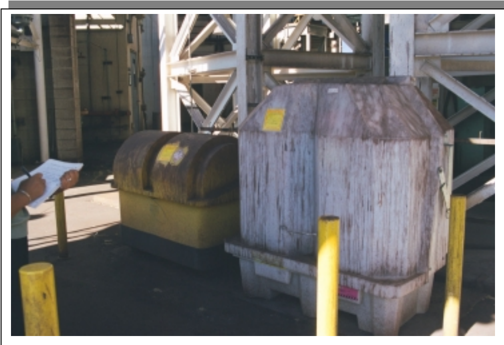
Satellite accumulation points at HATS with rust stains.
