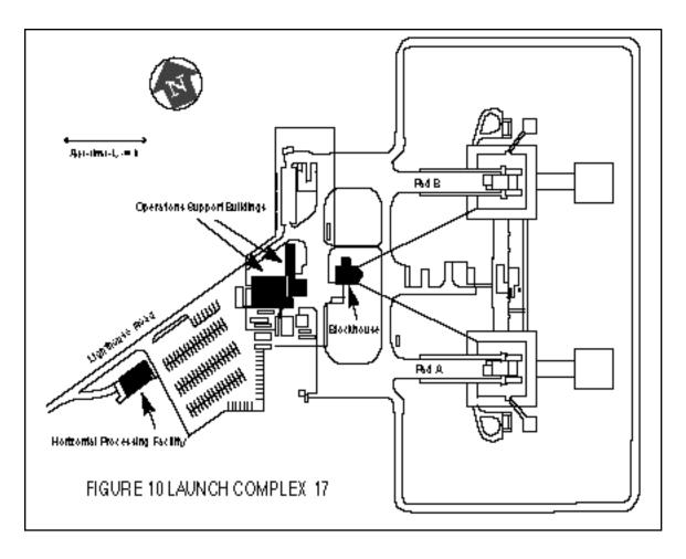
Launch Complex 17 (LC-17). At the HPF, the first stage destruct ordnance will be installed and the first stage prepared for erection on one of the two launch pads at LC-17. At the launch pad, the first stage will be erected and secured for assembly with the remaining parts of the launch vehicle.
