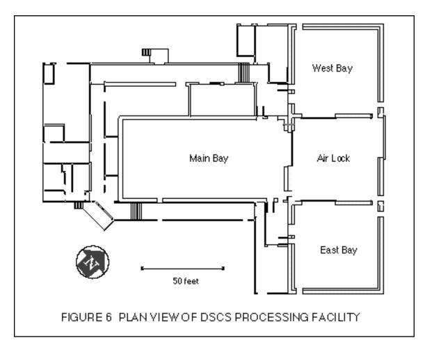
main processing facility for Block IIR SVs. Figure 6 is a plan view of this facility.
