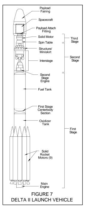
**Solid Rocket Motors.** Nine solid rocket motors are attached to the first stage engine section to provide additional thrust. These
