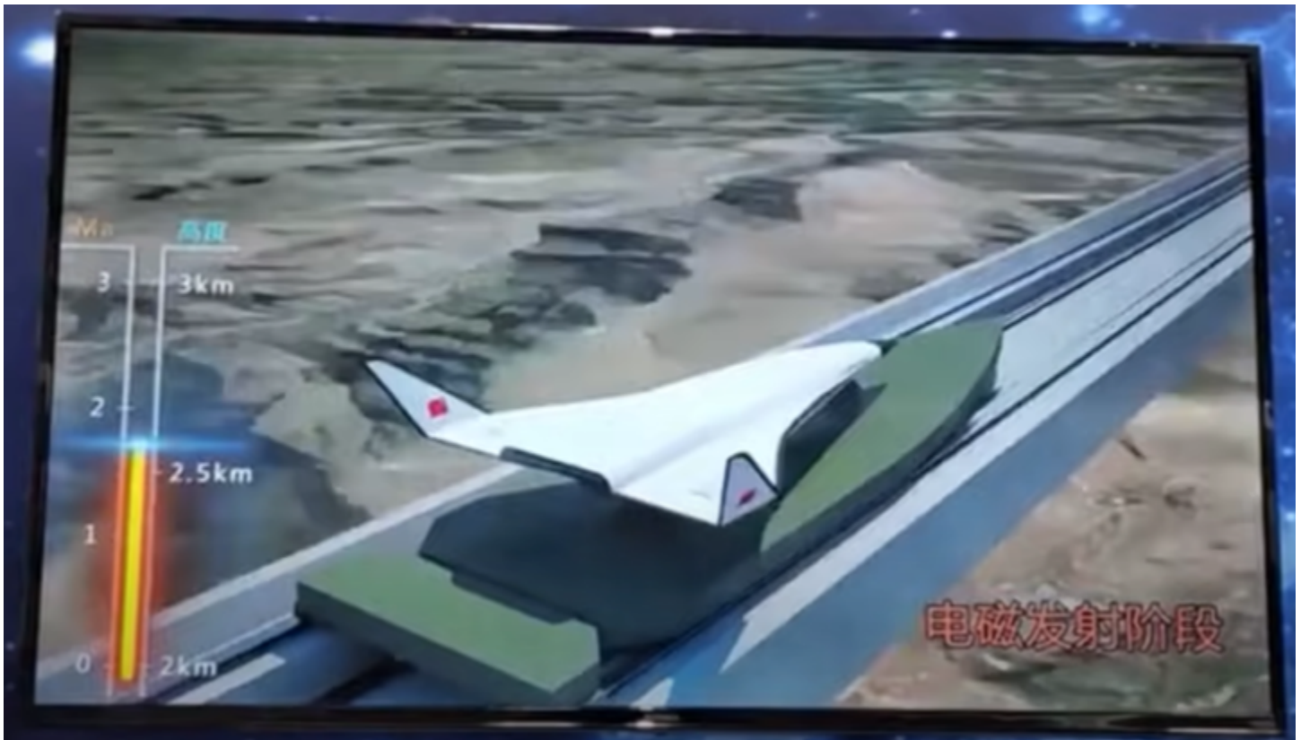
A screenshot from a CALT presentation showing a rail launched HTHL spaceplane.
