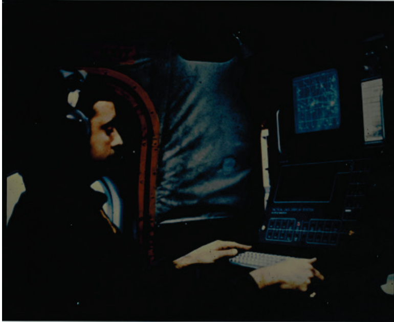
Figure 18. An Outlaw Shark terminal installed in a Navy EP-3 aircraft
