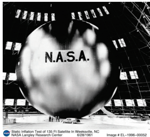
Figure 4. Echo satellite sphere, used by the Navy for pioneering satellite communications
