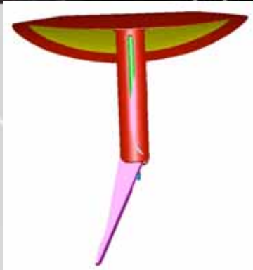
Plug development for on-orbit RCC repair led by Langley
