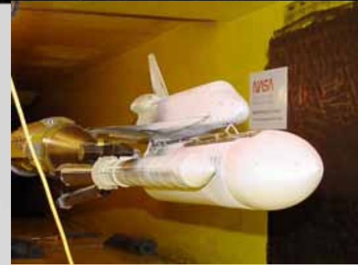
Shuttle 3% model tested in the Ames 9X7 supersonic wind tunnel
