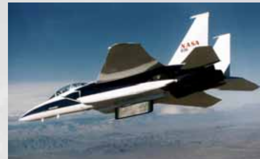
ET foam flight testing Dryden Aerodynamic Flight Test Fixture on F-15B aircraft
