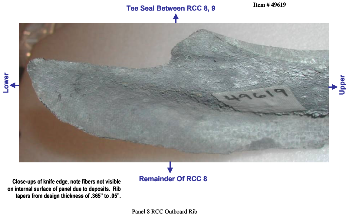
Figure 5-4. Example of rib erosion
