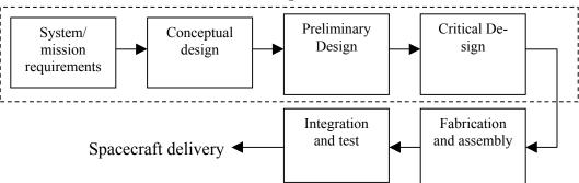
Fig. 10-1 Spacecraft design phases
