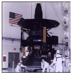
Fig. 10-8 NASA Galileo Spacecraft with two nuclear powered generators
