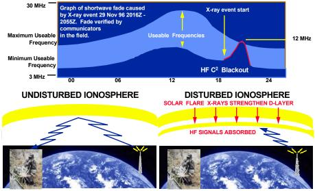
Fig. 6-5. High Frequency (HF) Propagation Windows
