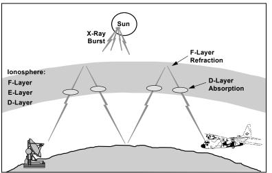
Fig. 6-4. High Frequency (HF) Communications
