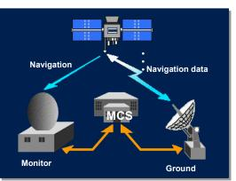
Fig. 14-5. Control Segment Interactions
