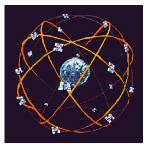
**Fig. 14-3. GPS Constellation** Most of the satellites in the constellation
