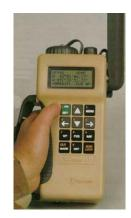
Fig. 14-9. Hand-held Precision Lightweight GPS Receiver (PLGR)
