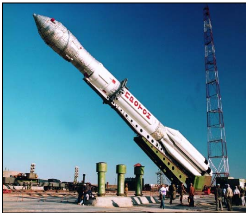
Fig. 20-10. SL-12 Lift to launch pad
