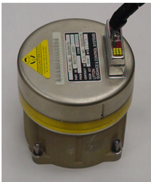
Figure A.1 LN-200 Fiber Optic Gyroscope
