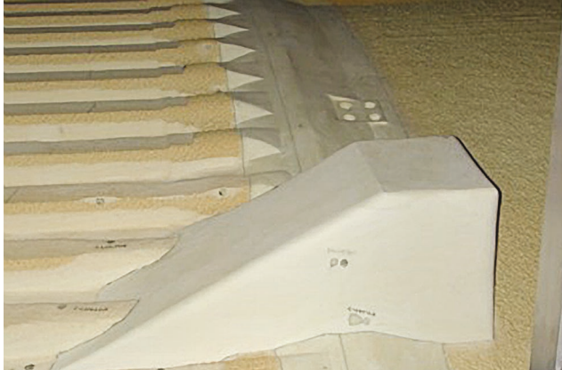
Figure 3.2-1-2. ET forward bipod ramp (foam).
