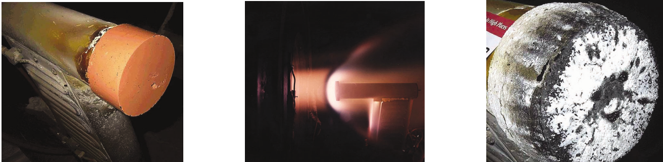
Figure 6.4-1-4. Tile repair material before, during, and after arc jet testing at 2300°F.
