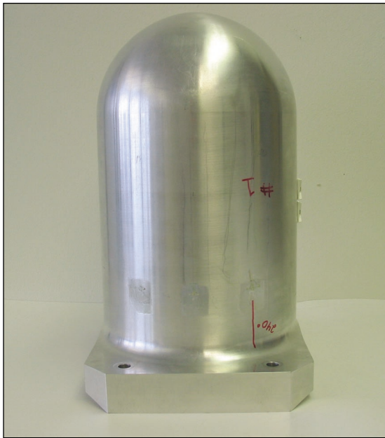
Figure 4.2-1-3. New one-piece forging design.
