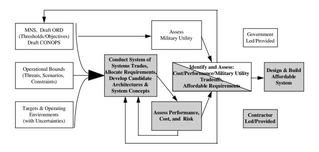
Figure 9. SBIRS Pre-EMD Process Flow
