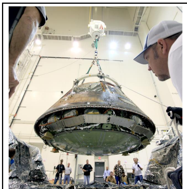
Inside the Launch Abort System Facility at NASA's Kennedy Space Center (KSC) in Florida, workers are preparing the Orion spacecraft that flew on EFT-1 in 2014 for transport to a laboratory to perform additional testing. The flown EFT-1 spacecraft is helping NASA finalize the Orion designs. Orion will next launch atop NASA's SLS rocket on EM-1)
