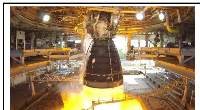
On January 9, 2015, RPT performed the first RS-25 engine on the A-1 test stand at SSC in Mississippi. This successful 300-second test began a multi-year testing effort required to prepare the engine for use on the SLS Core Booster Stage..
