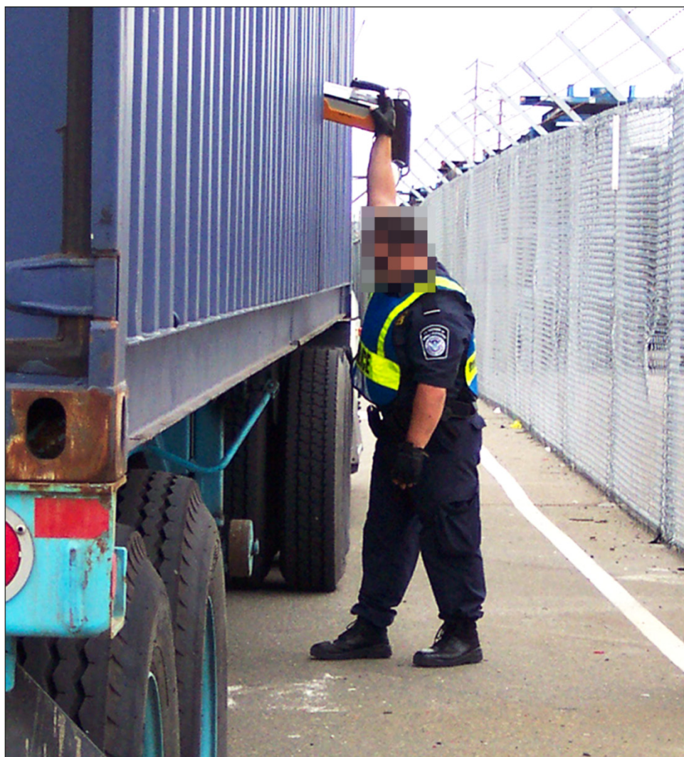
Figure 2: CBP Officer Screening a Truck with a Handheld Detector That Can Identify Sources of Radiation
