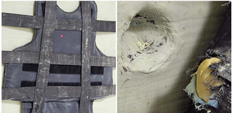
Figure 2: Ballistic-Resistant Body Armor Mounted on Clay for Testing Purposes
