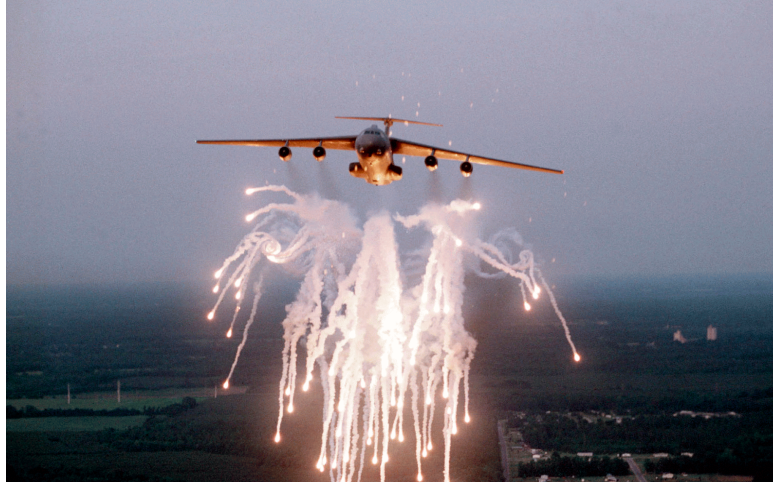
Figure 2: C-141B Starlifter Ejecting Flares on Takeoff
