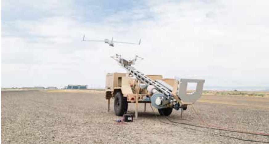
A ScanEagle unmanned aerial vehicle takes off from its pneumatic launcher. (SIGAR photo)
